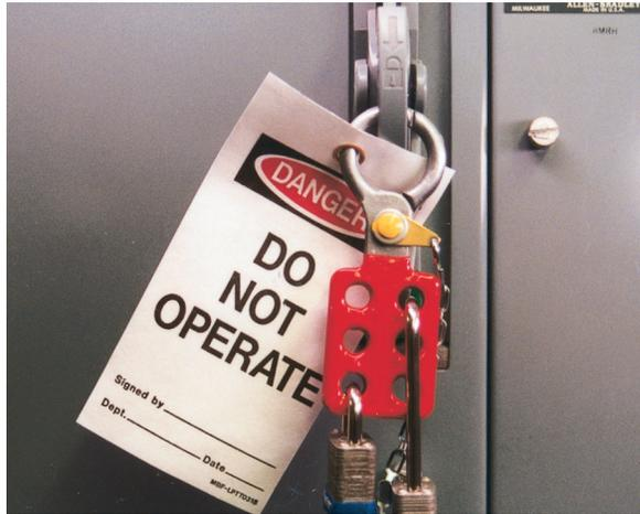
**FIGURE S-5** The equipment can be locked out by several different people.
